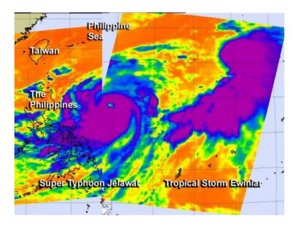
This combined image was created from infrared AIRS data of Super Typhoon Jelawat on Sept. 25 and Tropical Storm Ewiniar on Sept. 24 to give perspective of their distance from each other. The eye of Jelawat is clearly visible in the middle of powerful thunderstorms (purple) with very cold cloud top temperatures. Credit: NASA JPL/Ed Olsen
