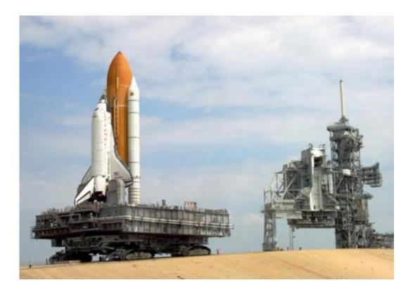
Shuttle Discovery riding one of KSC's crawler-transporters to Launch Pad 39B in June 2005 (NASA)
