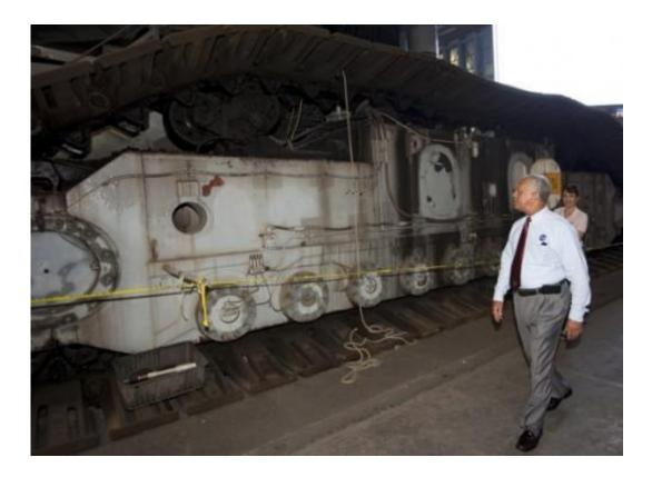
In addition to carrying capacity CT-2 will also be getting new brakes, exhausts, hydraulics and computer systems.
