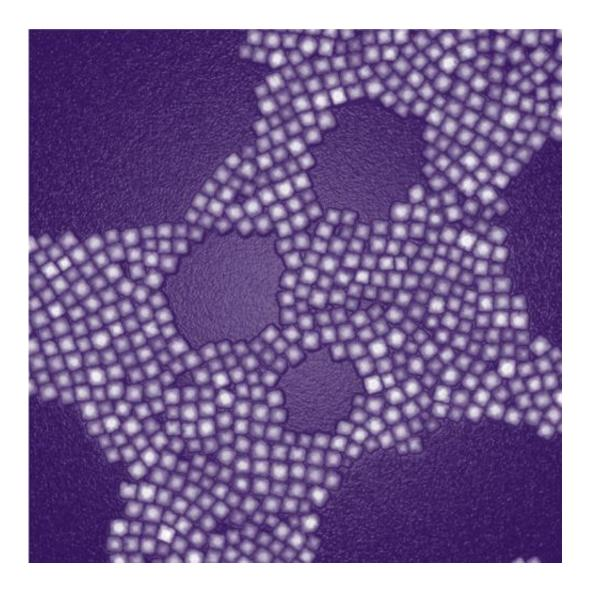
This is a transmission electron microscopy image of nanoparticles designed for deep-tissue imaging. Each particle consists of a core encased inside a square, calcium-fluoride shell. Credit: Zhipeng Li
