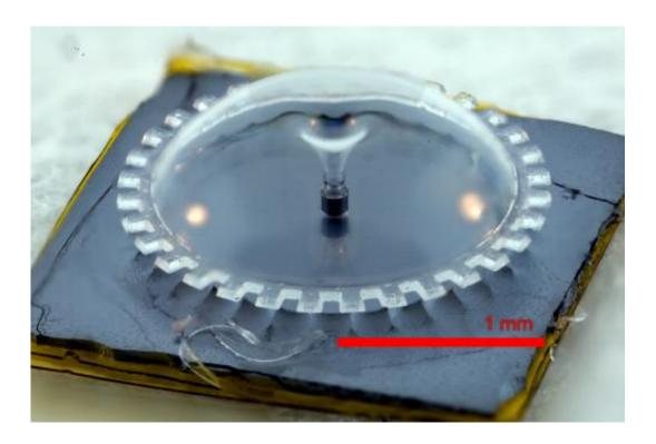
**Atomic layering of diamond**. Layering diamond over a blown structure or depositing CVD diamond in a micro-well on the substrate have been shown to be effective, promising methods for creating highly symmetric, accurate 3-D inertial-sensor structures. Credit: University of California, Irvine
