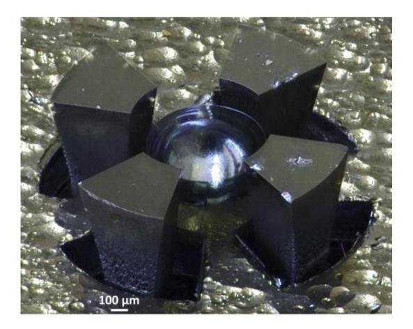
**Blown quartz**. Similar to glass blowing, quartz blowing can be used to make an even more symmetric structure. Researchers developed fabrication techniques
