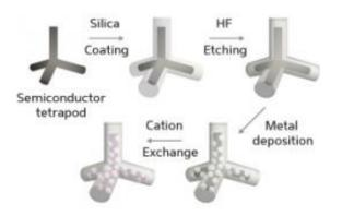
The water-based synthesis and cation exchange reaction of a platinum-decorated semiconductor tetrapod with a hollow silica shell. Credit: Ref. 1 © 2012 American Chemical Society
