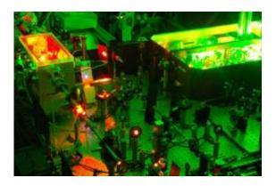
Laser system for generating ultra short x-ray pulses used in the experiment to make the recordings. Copyright: CAU, Photo: Rohwer et al.
