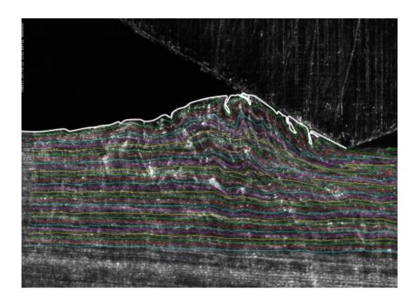
This frame from a high-speed camera sequence reveals surprising behavior in a solid piece of metal sliding over another. The research is providing new insights into the mechanisms of wear and generation of machined surfaces that could help improve the durability of metal parts. A publication-quality image is available at https://news.uns.purdue.edu/images/2012/chandrasekar-metals.jpg Credit: N. Sundaram and Y. Guo
