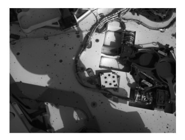
This set of images from NASA's Curiosity rover shows the inlet covers for the Sample Analysis at Mars instrument opening and closing, as the rover continues to check out its instruments in the first phase after landing. These images were taken by the Navigation camera on the 36th Martian day, or sol, of the rover's operations on Mars (Sept. 11, 2012). The rover's mast is casting a shadow over the deck. Image credit: NASA/JPL-Caltech
