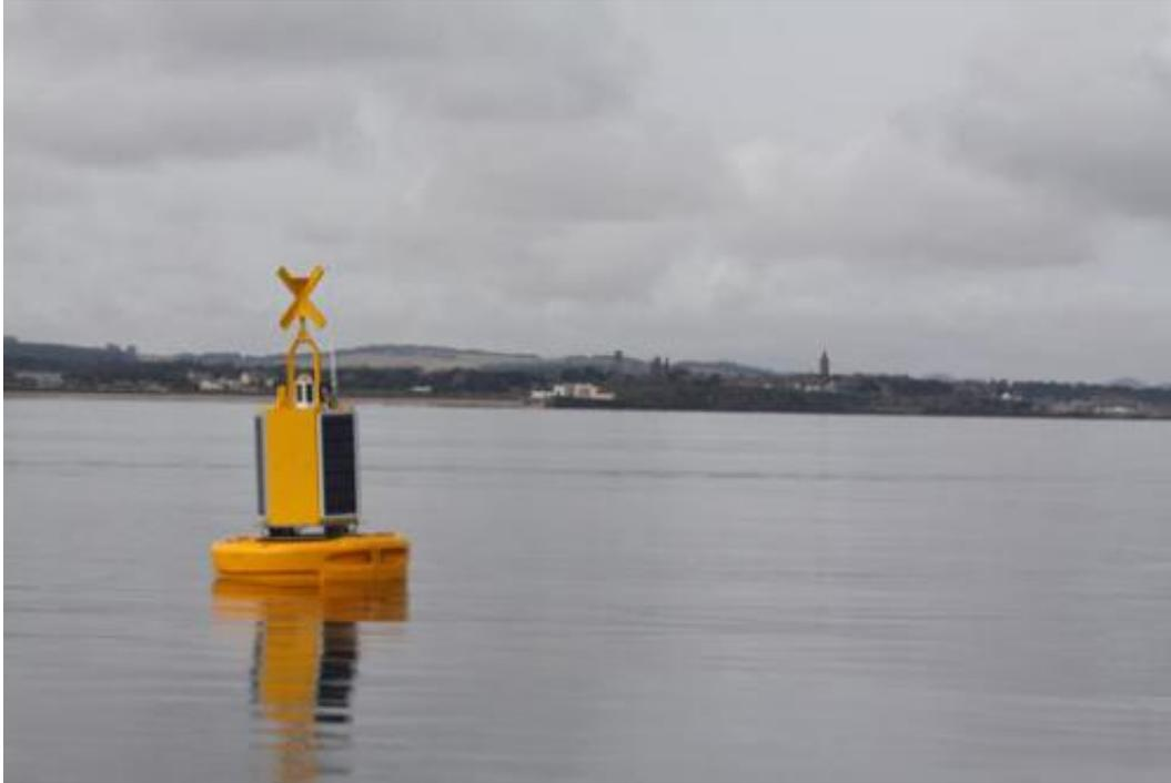
PAMBuoy, a new instrument to detect whales, dolphins and other marine mammals, and provide immediate alerts during the development of offshore wind, wave and tidal installations.
