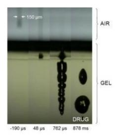
To test the effectiveness of the drug delivery system, a special gel is used to mimic the behavior of human skin. Here the jet first creates a hole on the surface of the gel, then, at a lower jet pressure, the drug is delivered into the skin. This gel simulation also reveals that there is no <code>?splashback?</code> from the injection, which is an important patient safety factor. Credit: *Optics Letters*
