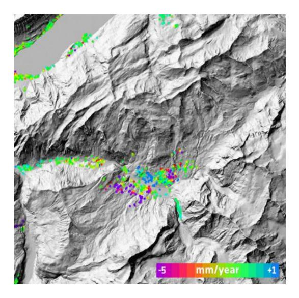
The Swiss village of Grindelwald in the Bernese Alps experienced slope movements on both sides of the valley during 1995–2000. Colours represent the average yearly displacement rates derived using radar data from ESA's ERS mission. Credit: ESA / Gamma Remote Sensing
