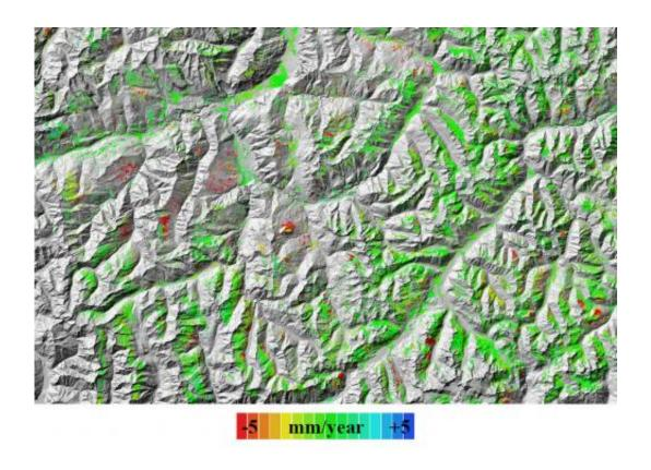
The Grison Alps in eastern Switzerland. The colours represent mean yearly displacement rates derived from Envisat data 2002–10. Red dots depict a subsidence of at least 5 mm per year. Credit: ESA / Gamma Remote Sensing
