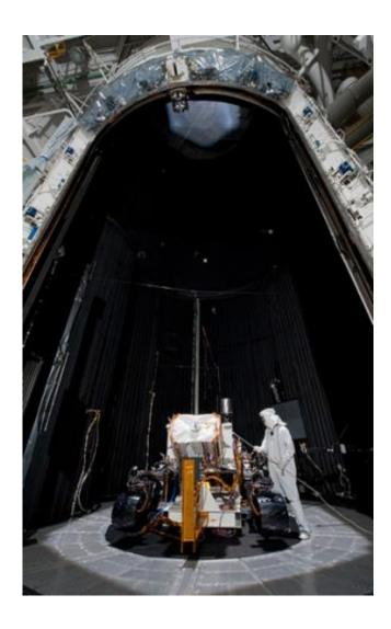
Curiosity, the Mars Science Laboratory rover, was prepped for pre-launch survival testing under Martian conditions in JPL's space simulator on March 8, 2011. The sealed chamber was pumped down to the near-vacuum of Mar's atmosphere, and chilled to –130°C by flooding its walls with liquid nitrogen. Credit: NASA/JPL-Caltech
