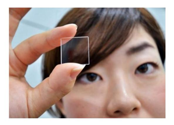
A woman holds up Japanese electronics giant Hitachi's new quartz glass plate technology, which can be used to store data indefinitely, in Tokyo on September 24. The company on Monday unveiled a method of storing digital information on slivers of quartz glass that can endure extreme temperatures and hostile conditions without degrading, almost forever.
