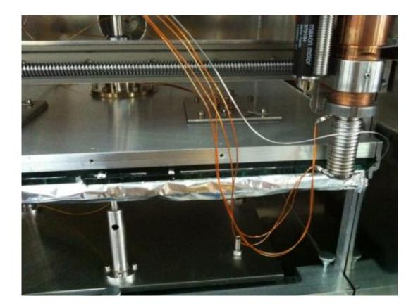
The experimental setup at Empa used to produce glazing prototypes with the new edge sealing technique. The cylindrical, copper-colored injection head is clearly visible - it injects a liquid tin alloy between the panes. Photo: Empa
