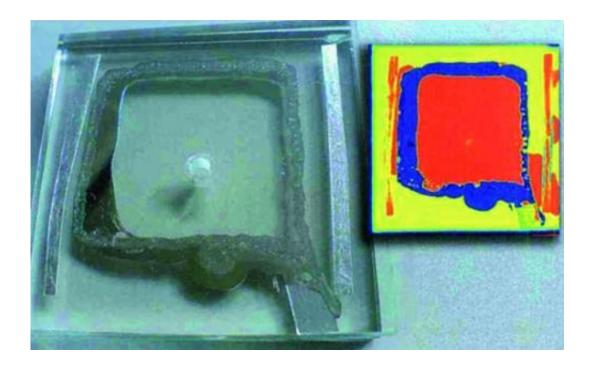
Vacuum glazing achieves very good thermal insulation. The challenge consists of sealing the panes of glass so well that the vacuum in the space between them persists over decades. Empa researcher have patented a method whereby the two panes are sealed with a tin-based alloy. The ultrasonic image of a laboratory experiment (right) shows that the bonding with the tin was successful throughout. The air-tightness was confirmed with leak measurements. Photo: Empa
