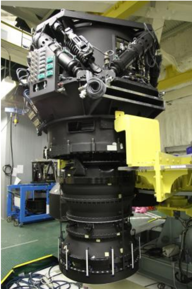
Hyper Suprime-Cam. The instrument weighs 3 tons and is 3 meters (9 feet) high. Credit: NAOJ
