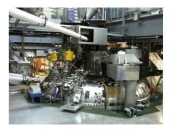
The Madison Symmetric Torus gained new capabilities with the installation of a neutral beam injector.
