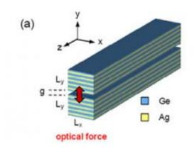
Missouri S&T researchers' modeling of stacked nanoscale slot waveguides made of metamaterials shows an optical force 100 to 1,000 times greater than conventional slot waveguides made from silicon.
