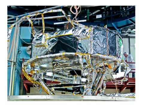
Close-up of Gaia's service module inside the SIMLES test facility at Intespace, Toulouse, during thermal balance and thermal–vacuum testing. The service module houses electronic units to run the mission's science instruments, and the units required to provide the spacecraft resources, such as thermal control, propulsion, communication, and attitude and orbit control. Credit: Astrium SAS
