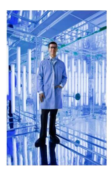
The state-of-the-art Environmental Chamber is used to study the aerosol lifecycle. The chamber is located in the Atmospheric Measurements Laboratory at PNNL. The purple glow is generated by ultraviolet lights that simulate the actions of sunlight. Scientists re-create atmospheric reactions in the chamber by injecting gas-phase aerosols and modeling their reactions.
