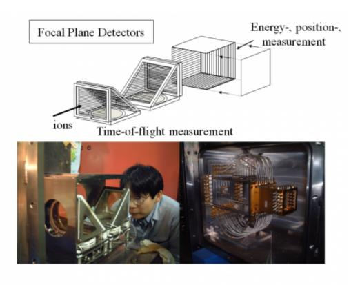
Figure three shows focal plane detectors. Credit: RIKEN
