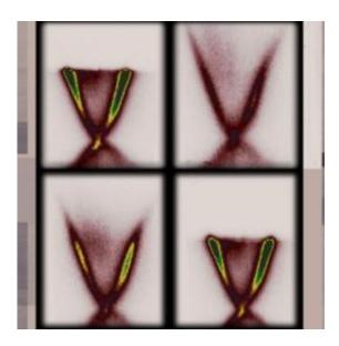
Three-dimensional graphical representations of the way electrons respond to an input of energy, delivered by a pulse of laser light. The horizontal axis represents the electrons' momentum, and the vertical axis shows their energy. The time sequence runs from top left to bottom right, and the laser pulse arrives just before the second image, causing a sudden burst of higher energy levels. Images courtesy of Yihua Wang and Nuh Gedik
