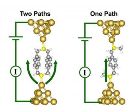
Atomic scale visualization of the single molecule junctions formed with two equivalent pathways (left) and one pathway (right), including the bonding to the tips of two gold electrodes and a schematic of the external electrical circuit.
