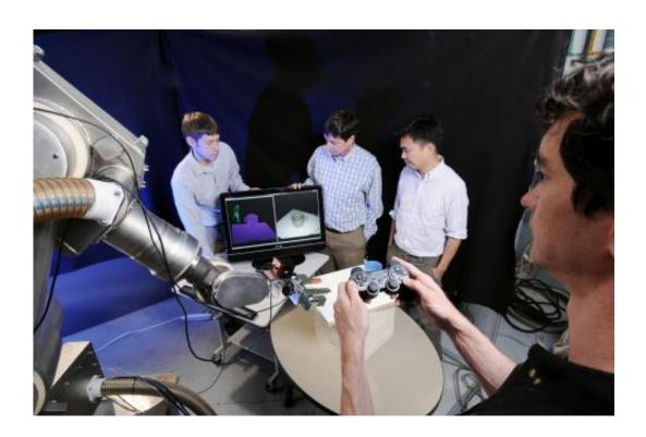
Matt Marshall, a Ph.D. student in the Georgia Tech School of Mechanical Engineering, uses a joystick controller based on visual servoing to command the motions of a robotic arm (with a 3-D camera attached) to grasp a cup. Shown left to right are Michael Matthews, a research engineer; Gary McMurray, a GTRI division chief; Ai-Ping Hu, a GTRI research engineer, and Marshall. Credit: Gary Meek
