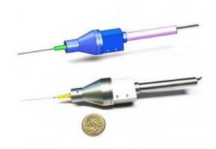
This shows the CAD model and prototype of the fiber-optic-sensor-based microsurgical tool, SMART. Credit: Courtesy Cheol Song, Johns Hopkins University
