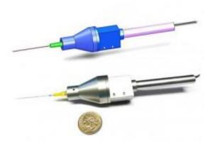
This shows the CAD model and prototype of the fiber-optic-sensor-based microsurgical tool, SMART. Credit: Courtesy Cheol Song, Johns Hopkins University
