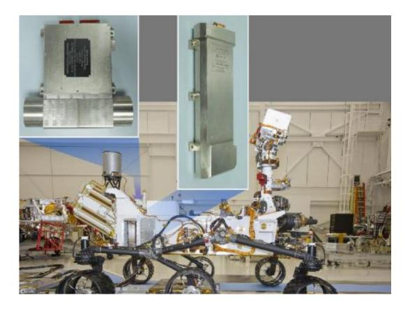
This image of NASA's Curiosity rover shows the location of the two components of the Dynamic Albedo of Neutrons instrument. The neutron generator is mounted on the right hip (visible in this view), and the detectors are on the opposite hip. Credit: NASA/JPL-Caltech
