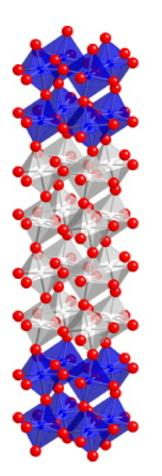
Illustration of a 4-unit-cell film of NdNiO3 (white) confined by LaAlO3 (blue) at the boundaries to make a quantum well structure.
