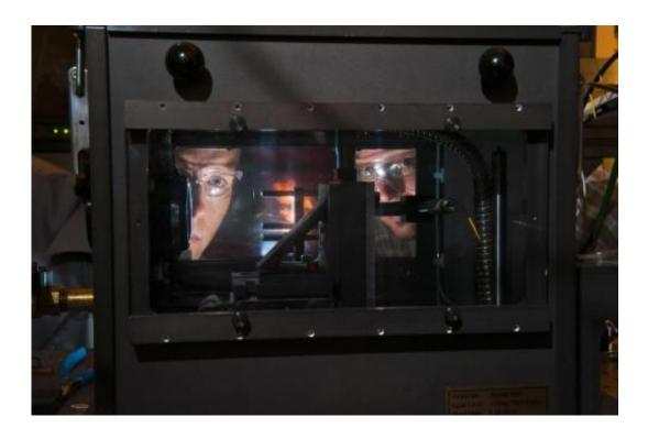
Sandia researchers Alex Tappan (left) and Rob Knepper watch the detonation of a critical thickness experiment. The experiment typically uses less explosive material than the size of one-tenth of an aspirin tablet to determine small-scale detonation properties. The bench-top experiment is so small, researchers can stand next to the firing chamber with eye and ear protection. Credit: Randy Montoya
