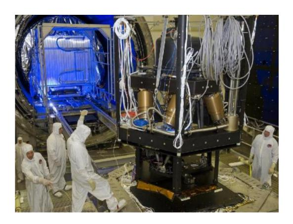
(Phys.org)—Testing of the James Webb Space Telescope's Center of Curvature Optical Assembly, or COCOA, recently was completed in the X-ray and Cryogenic Test Facility at NASA's Marshall Space Flight Center in Huntsville, Ala. The optical assembly was operated in a vacuum at both room temperature and cryogenic—or deep cold—temperatures to certify its performance before it is used to test the
