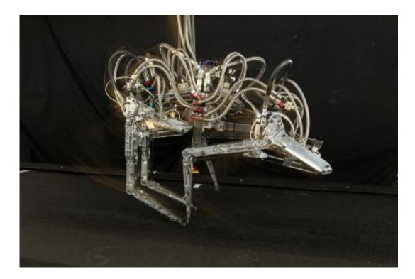
(Phys.org)—DARPA's Cheetah robot—already the fastest legged robot in history—just broke its own land speed record of 18 miles per hour (mph). In the process, Cheetah also surpassed another very fast mover: Usain Bolt. According to the International Association of Athletics Federations, Bolt set the world speed record for a human in 2009 when he reached a peak speed of 27.78 mph for a 20-meter split during the
