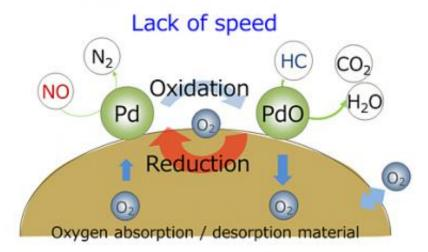
Since palladium(Pd) lacks performance in purification of exhaust emissions, rhodium is needed to complete this process.
