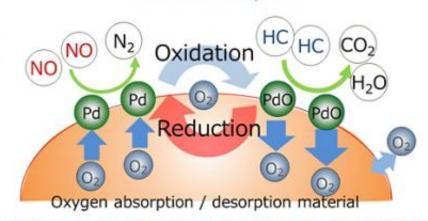
Enhance performance of palladium (Pd) in purification of exhaust emissions to replace a portion of rhodium use.
