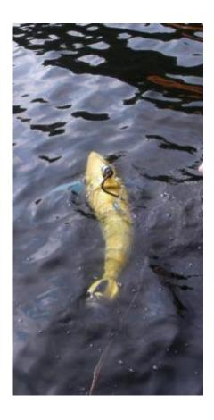
This shows BIOSwimmer? in the water during testing. Note the line seen is a tether for the camera, not for the fish. Credit: Boston Engineering Corporation?s Advanced Systems Group in Waltham, Massachusetts
