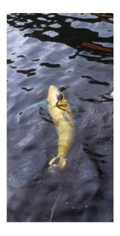
This shows BIOSwimmer? in the water during testing. Note the line seen is a tether for the camera, not for the fish. Credit: Boston Engineering Corporation? Advanced Systems Group in Waltham, Massachusetts
