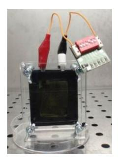
A lab-scale microbial fuel cell, used to study the generation of electricity from waste products. Credit: Lisa Buddrus
