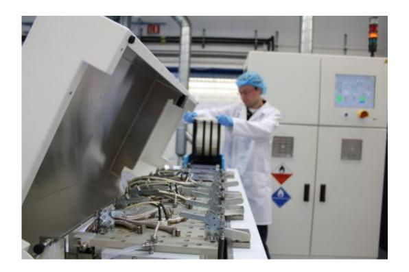
SoLayTec InPassion LAB (PDT) tool for deposition of spatial ALD Al2O3.
