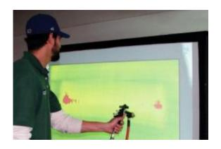
A spray-paint technician in training uses VirtualPaint, a painting simulator designed to teach military personnel, commercial painters and other paint spray technicians the correct techniques for spray paint operations. Credit: IWRC and Ames Laboratory -- USDOE
