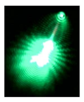
Laser light is emitted from the end of a cadmium sulfide nanowire.
