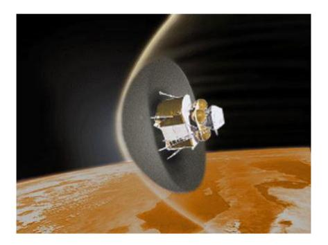
An artist's concept of a spacecraft using a heat shield made from the soil of another world, called regolith. Credit: NASA
