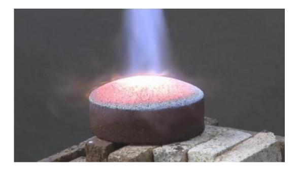
A 2-inch by 4-inch brick is heated by a welding torch in a test of a concept for making heat shields from the soil of other worlds. Credit: NASA
