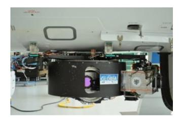
The GLORIA infrared spectrometer after installation underneath the body of HALO. Credit: Mahesh K. Sha, KIT
