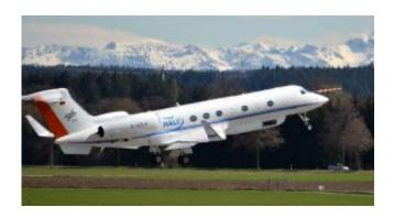
HALO is taking off. The "bellypod" that accommodates the GLORIA infrared spectrometer can be seen underneath the aircraft fuselage. Credit: Mahesh Kumar Sha, KIT
