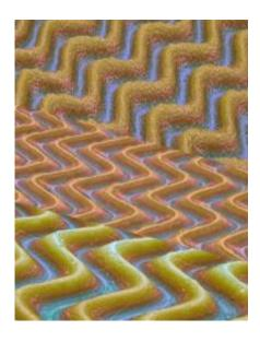
Images taken with a 3-D microscope show wrinkled surfaces produced using a method developed by the MIT team. The size, spacing and angles of the wrinkles vary depending on how much the original underlying surface was stretched, and how the stretching was released. Images by Jorge Luis Yague and Felice Frankel
