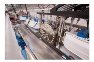
To create a precise X-ray band and make the Linac Coherent Light Source even more "laser-like," researchers installed this chamber with a slice of diamond crystal. The new hardware sits halfway down the 130-meter bank of magnets where the X-rays are generated. Credit: Photo by Matt Beardsley, SLAC National Accelerator Laboratory
