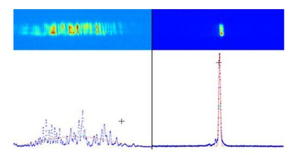
The LCLS's new self-seeding improvements yield laser pulses focused to higher intensity in a much narrower band of X-ray wavelengths, as you can see in these spectrographs comparing a normal SASE (self-amplified spontaneous emission) pulse (left) and a seeded one (right). The results promise to speed research discoveries and may enable experiments that have never before been possible. Credit: Graph from J. Amman, et al. adapted by Greg Stewart, SLAC National Accelerator Laboratory
