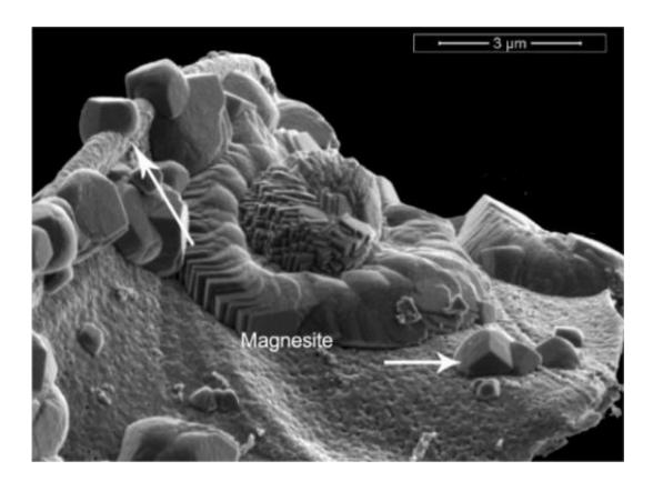
High-resolution scanning electron microscopic images of the reacted forsterite indicating the formation of magnesite (cubes).
