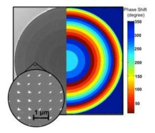
Left: A micrograph of the flat lens (diameter approximately 1 mm) made of silicon. The surface is coated with concentric rings of gold optical nanoantennas (inset) which impart different delays to the light traversing the lens. Right:The colored rings show the magnitude of the phase delay corresponding to each ring. (Image courtesy of Francesco Aieta.)
