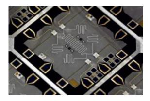
The device in the photomicrograph was used to run the first solid-state demonstration of Shor's algorithm. It is made up of four phase qubits and five superconducting resonators, for a total of nine engineered quantum elements. The quantum processor measures one-quarter inch square. Credit: UCSB
