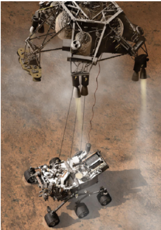
A rocket-powered sky crane lowered the rover to the ground dangling from a cable. (Image by NASA/JPL)
