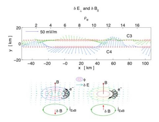
The electric field forms vortices propagating past two of the Cluster spacecraft. Since the electrons have much lower mass than the ions and can easily be moved around by the electric field, the electrons create a magnetic field, as shown in the bottom panel. (Fig. from Norgren et al., PRL, 2012)
