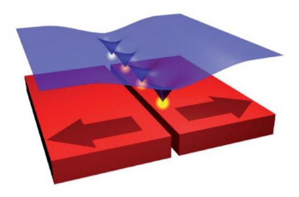
A schematic diagram shows Majorana particles as they might line up in two opposing magnetic fields (red) that interact with a superconducting topological insulator (blue). (Reprinted with permission from Neupert, Onoda, and Furusaki, PRL 105, 206404 (2010) (http://dx.doi.org/10.1103/PhysRevLett.105.206404); Copyright, the American Physical Society.)
