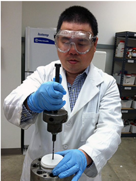
Associate Professor Zhengdong Cheng opens the autoclave where the ion exchanger crystals are produced. The ion exchangers will then be paired with a pH-sensitive hydrogel to create oscillating drug-delivery particles.
