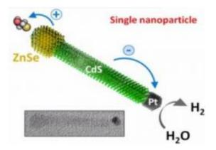
This is a schematic of the photocatalytic nanocrystal. Credit: *Journal of Visualized Experiments*
