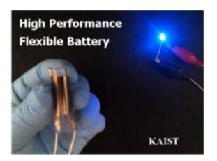
This shows a blue LED emission operated by flexible solid state battery. Credit: Korea Advanced Institute of Science and Technology
