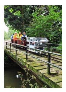
Engineering students and staff at the University of Birmingham have designed and built a prototype hydrogen powered locomotive, the first of its kind to operate in the UK.
