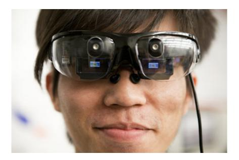
Chuck Yang, M.Eng. '12, models a pair of glasses that mirror a computer screen, providing the user with a heads-up display as he communicates with a robot on a search-and-rescue mission. Image: Lindsay France
